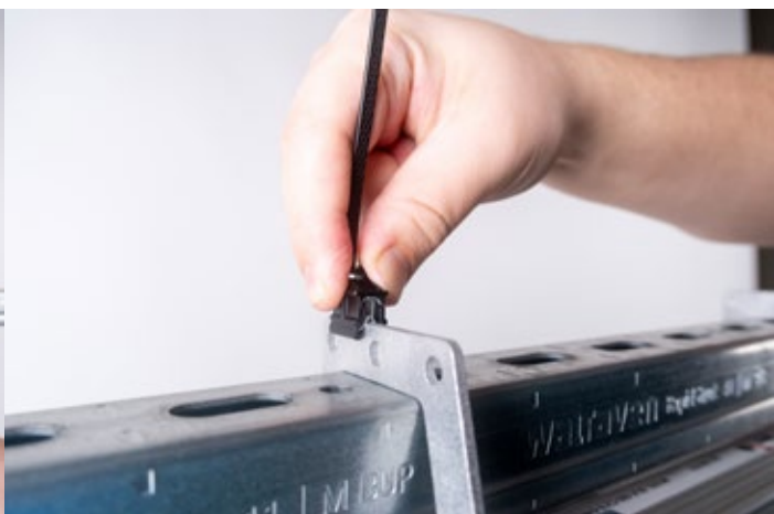
Step 10: Place them on the LED driver hanging brackets
